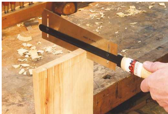
▲ Pic.9 Cutting finger joints with the rip side of a specialist ryouba with very fine teeth
